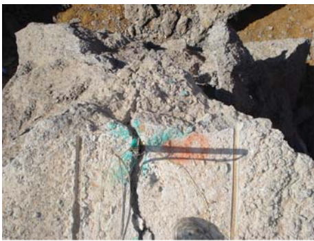
Figure 6. Final fracture pattern of cube 1 looking directly over borehole.
